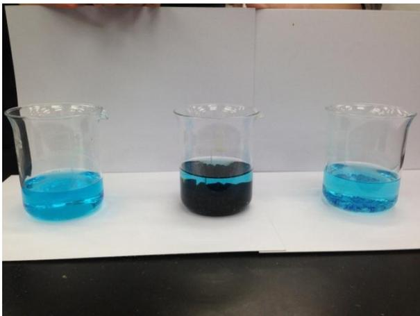
(From the left, before treatment, after active carbon treatment, and after photocatalytic treatment)
